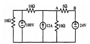
**SOLUTION:** Using source transformation the equivalent circuit is,
