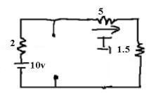
Solving parallel resistors (2//6)  $\frac{2\times6}{2+6} = 1.5\Omega$
